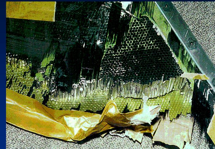
Enhanced diffusion along interface due to low cross-link density
