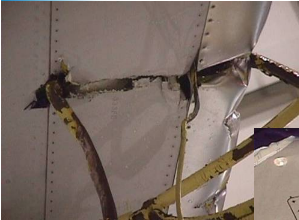
Skin/Spar Damage—Ground Handling Equipment Impact
