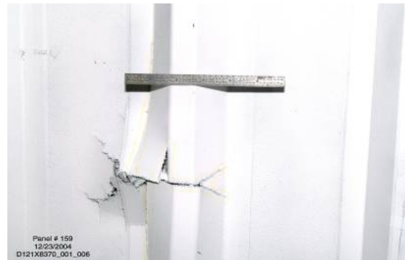
Inside damage associated with OML VID
