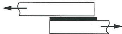
e. Adhesive Failure (Shear)
