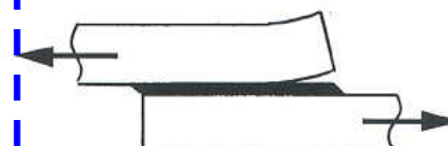
f. Adhesive Failure (Peel)
