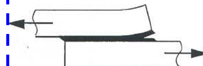
d. Cohesive Failure (Peel)
