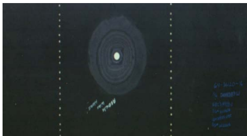
Lost Bonded Repair Patch
