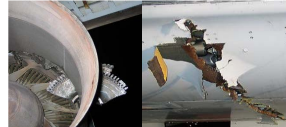
Rotor Disk Cut Through the Aircraft Fuselage Belly and Wing Center Section to Reach Opposite Engine
