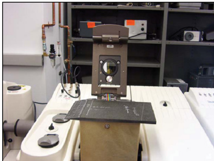
Figure 1. A composite sample placed on top of the integrating sphere module and ready for analysis
