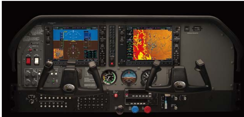
Figure 1: Cockpit of a Cessna 182 equipped with the Garmin G1000. Courtesy of Cessna Aircraft Company.
