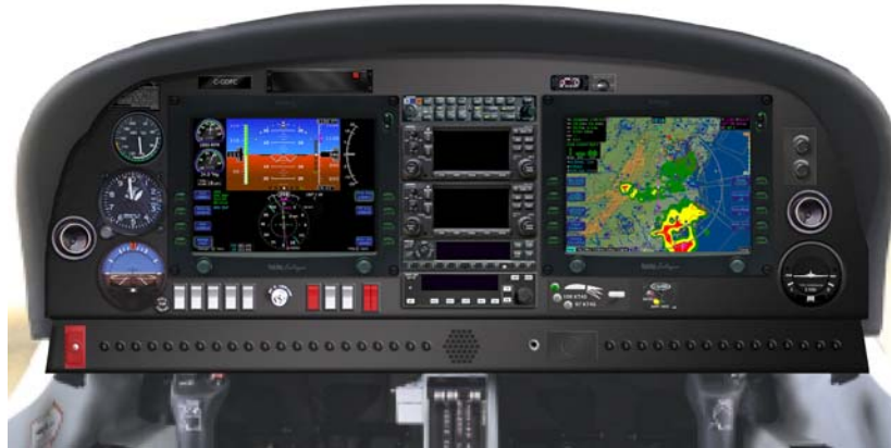
Figure 2: Cockpit of a Diamond DA40 equipped with an Avidyne Enterga suite. Courtesy of Avidyne Corporation.
