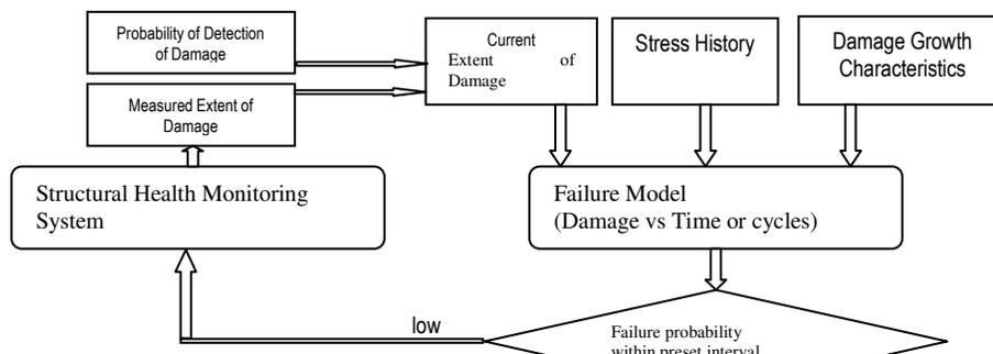
Fig. 7: Flow diagram of a structural health monitoring system
